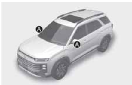
[A] Wide-side view camera (camera located at bottom of the mirror)
